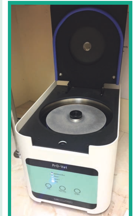
Figure 3: A blood centrifuge separates whole blood into its component parts
