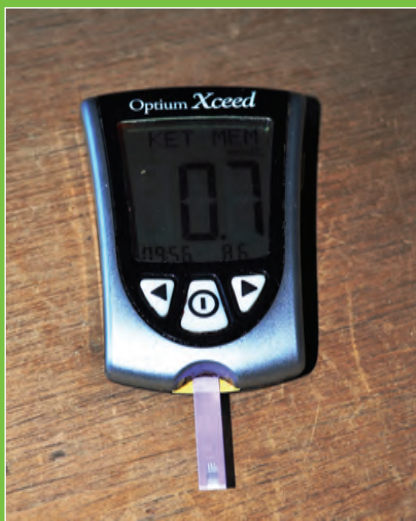
Figure three. A ketone meter is used to measure blood level of BHB in cows 4 days post-calving
